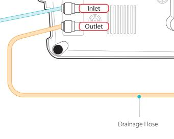
Make sure all connections are secure. Open the main valve and turn the power on. Make sure to use <u>cold water</u> to operate the unit.
