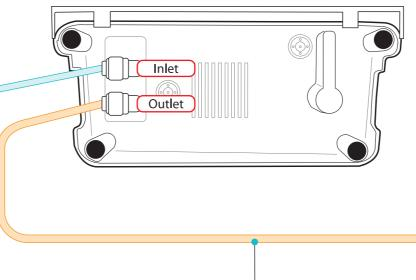
Remove the nut on the side of the tap water adapter. Connect the hose (1/4") to the adapter.
